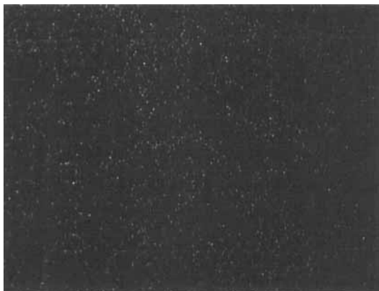
FIGURE 8. Optical micrograph taken at ambient temperature under polarised light of the cured 60/40 PDLC composition based on the bifunctional epoxy resin. Magnification 160X.
